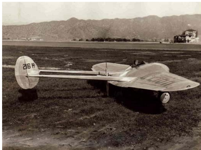
"Flying Wing" plane tested in California. An all-metal plane of radically different design can do over 100 miles per hour.
